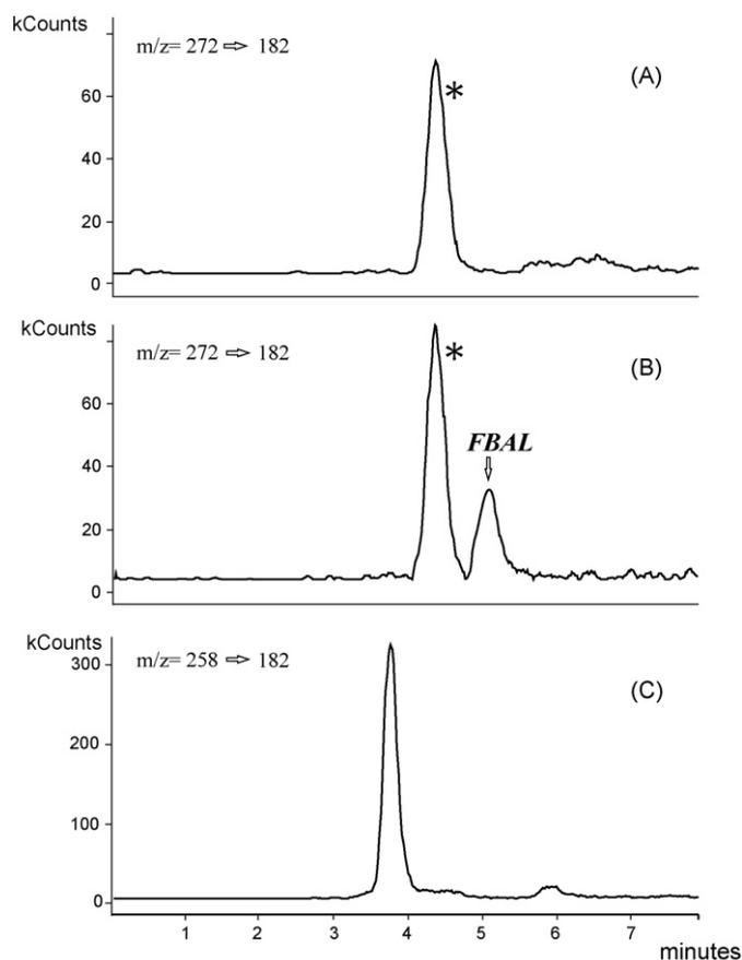
Fig. 3. MRM chromatograms for DNB-FBAL from blank human urine (A), auxiliary nurse exposed to 5-FU urine, FBAL concentration:  $2.30\ \mu\text{g/l}$  (B) and the internal standard (C). \*Urine impurity.
